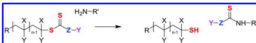
Scheme 18. Processes for RAFT End-group Transformation based on use of a functional RAFT agent to facilitate by-product removal (167).
