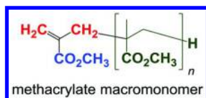
Figure 2. Structure of methyl methacrylate “macromonomer”
